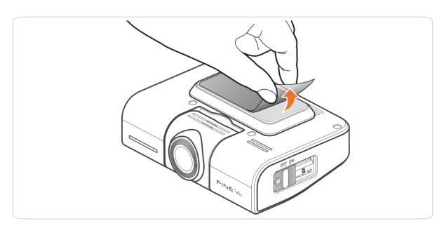
3. Peel off the protective film from the tape for attaching the cradle.
